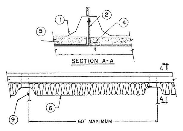
1. **Metal Roof Deck Panels\*** — 24 MSG min coated steel. Panels continuous over two or more spans. End laps to occur adjacent to purlin with panels overlapped 3 inches. A line of sealant may be used at panel ends and side laps. Adjacent panels to be seamed together along side using an electric seaming tool. Seaming operation to include panel clip tabs (Item 2).
